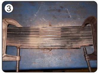
Lay springs on flat surface & install (2) C clamps.
