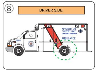
Reinstall spring pack in vehicle with new u-bolts,top plate and nuts as per workshop manual.
