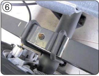
Enlarge hole on top plate to allow for clearance of nut. Enlarge to 3/4" using bit.
