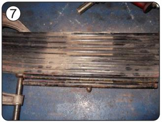
Install new center bolt into spring pack. Tighten nut properly and cut excess of bolt with die grinder.
