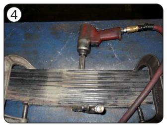
Remove spring center bolt (through bolt) with clamps installed (note: may require vice grips on bottom to hold through bolt while removing upper 15mm nut on through bolt).
