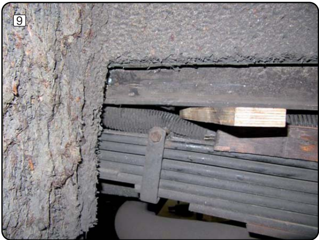
Make sure the heater hose is out of the way before drilling.
