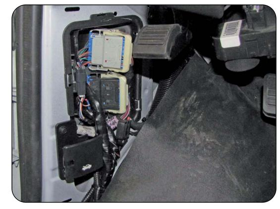
Locate and remove the circuit breaker on the red / black wire (F.ALT)
