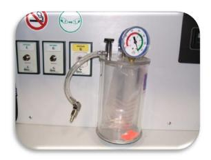
Turn thumb screw counter clockwise to remove canister
