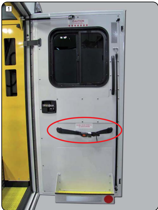
1 - Locate and remove the retaining strap for stair chair.
