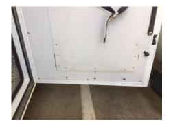
2. Install current Stair Chair Bracket with the supplied spacer kit and hardware, shown below.(apply one drop of blue thread Loctite to each supplied screw)
