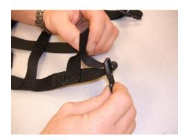
2) Use an appropriate heating device to safely seal the end of the cut strap
