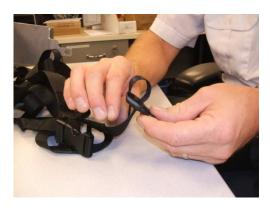
4) Install the pointed belt stop button to the end of the strap
