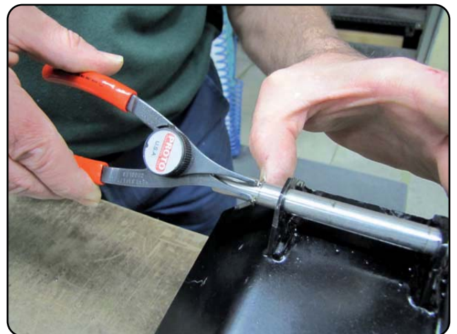
Install the retaining ring using appropriate tool as shown.
