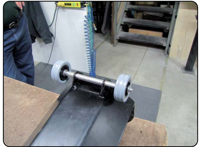
Install the retaining rings, washers and wheels. (See drawing 1.0).
