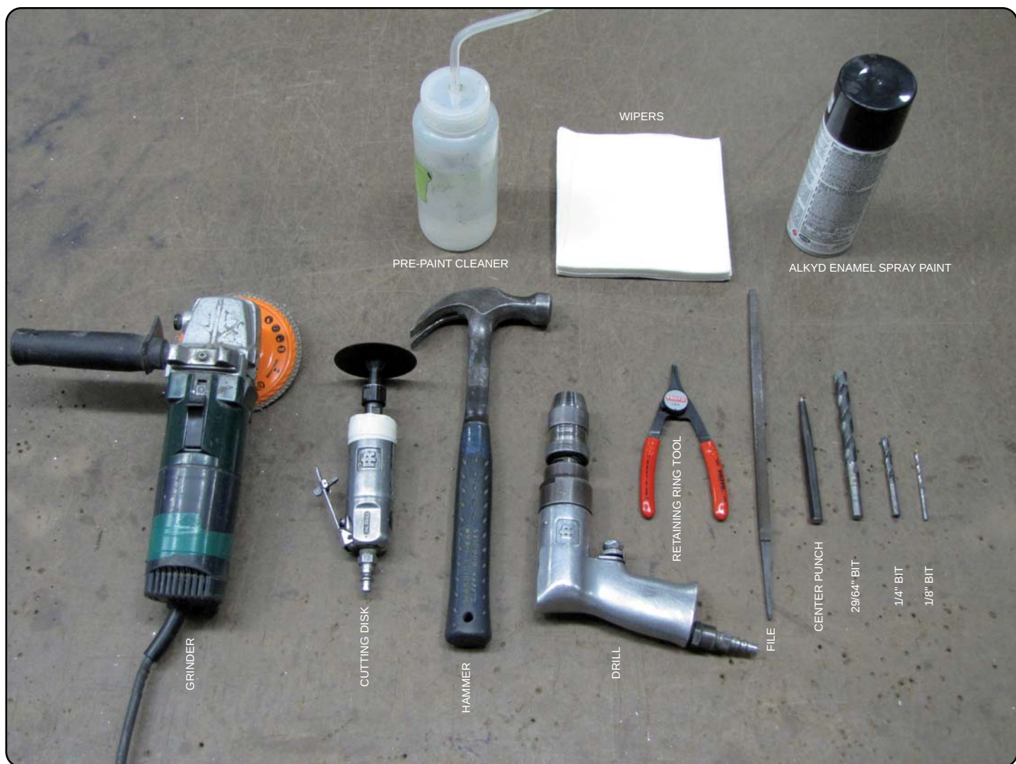
Necessary tools required to make the modification.
