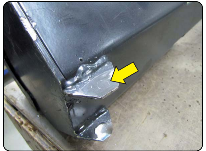
You should see where the axle used to be, and use that to mark the center of the new hole.
