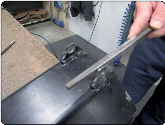
Use a file to remove sharp edges.
