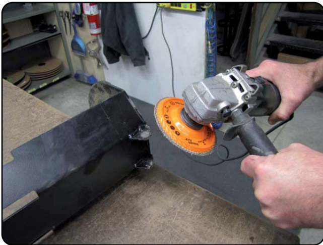
Use a grinder to remove the weld.
