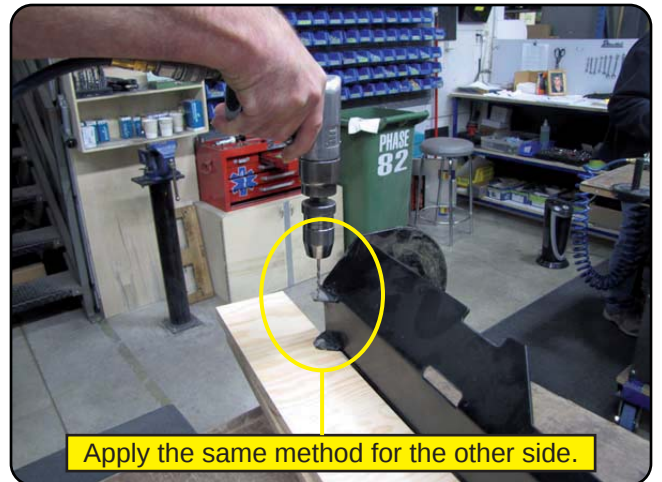
You should see where the axle used to be, and use that to mark the center of the new hole.
