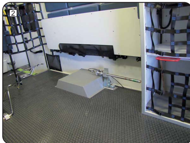
Actual setting of second stretcher release system.
