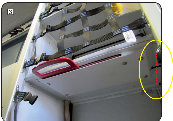
Cut the sheath and cable here.
