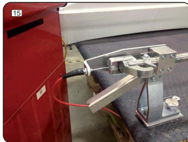
Insert the cable and the sheath as shown. Lock the cable in place as tight as possible with the stretcher arm in close position.
