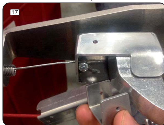
Reinstall small finishing aluminium piece with rivets.
