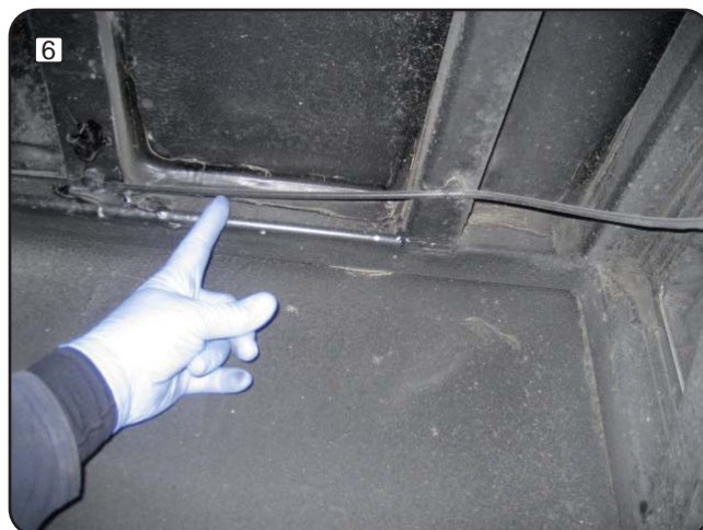
Remove the holding clips holding the old sheath. (Make sure to notice the course of the sheath).
