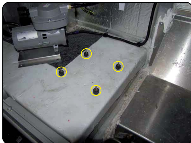
Manually install the rubber bushings in the holes.
