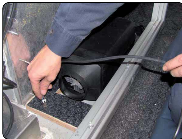
Pass the fuel metering pump power harness through the new hole.
