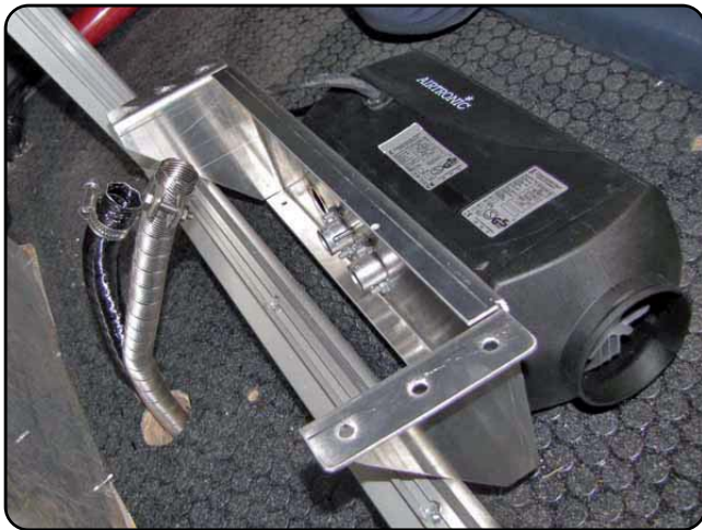
Disconnect the combustion air inlet and the exhaust outlet.
