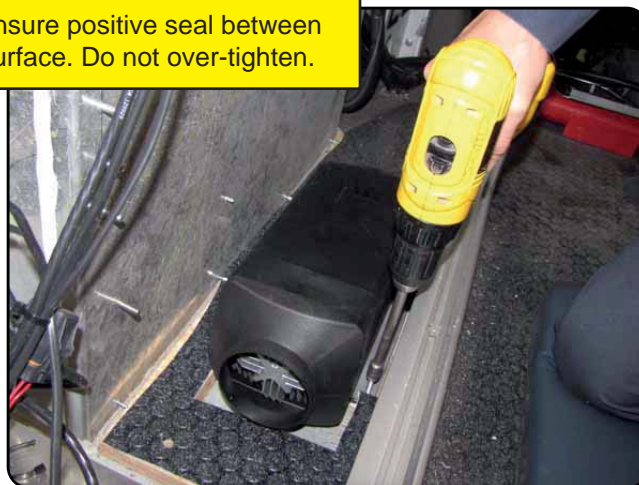
Use 4 provided screws to fix the air heater on the floor.
