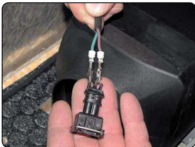
Remove the terminals on the connector from the fuel metering pump power harness.
