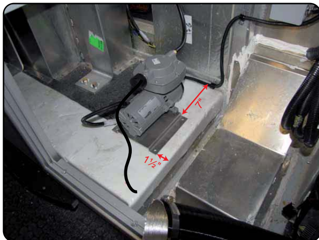
Place the suction pump as shown on picture to mark the new holes.
