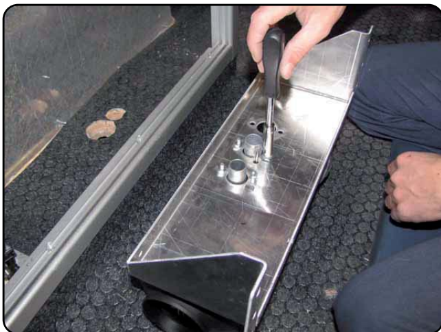
Remove the 4 nuts to remove the air heater from the support.
