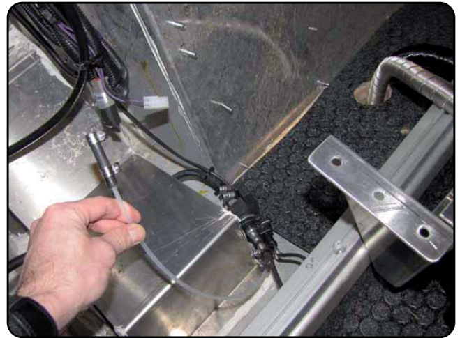
Remove the fuel metering pump hose. Send the fuel metering pump hose under the vehicle back through the floor.
