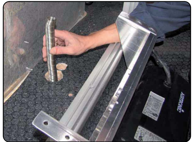
Send the combustion air inlet and the exhaust outlet under the vehicle back through the floor.
