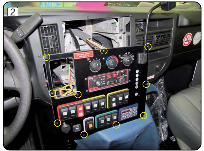
To remove the console panel, locate and unscrew the ten (10) screws as shown.
