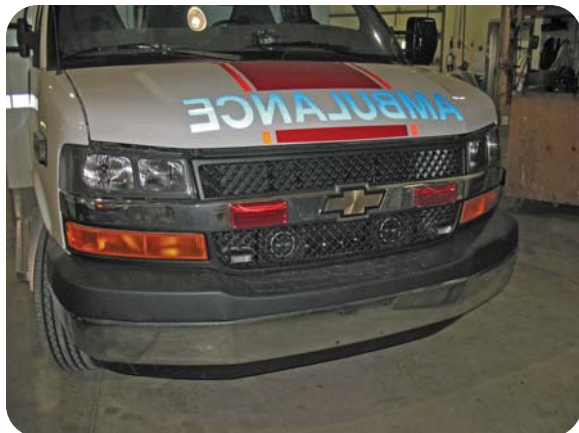
Remove the GM front grille to have access to the speakers.
