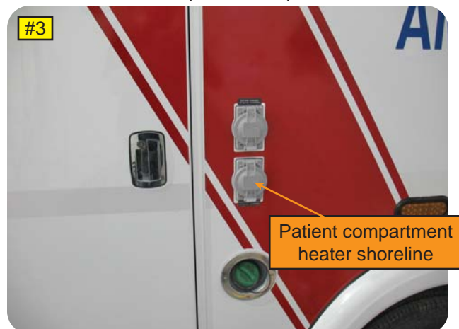
The patient compartment heater shoreline is located on the left side (driver side) of the vehicle.
