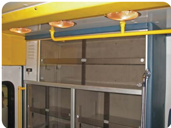
Remove the two (2) cabinet windows.
