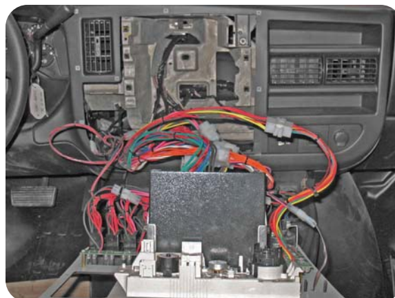
Remove the front console to have access to all connectors.
