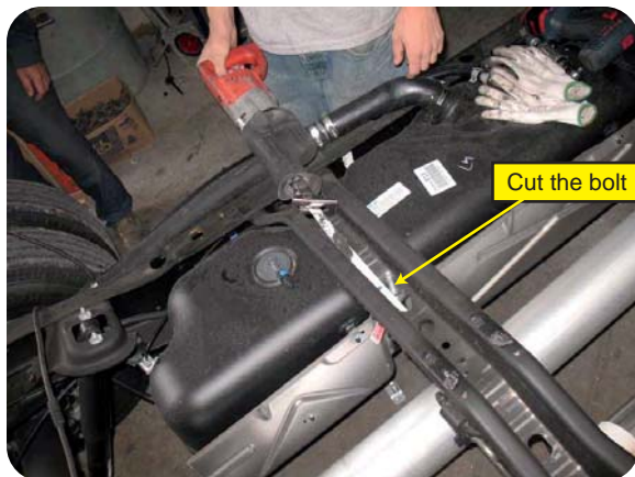
Cut the top of the bolt holding fuel tank.
