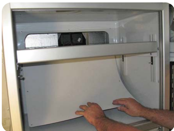
Remove the access panel.
