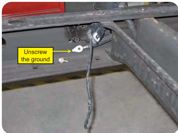
Unscrew the ground on the rear left side.
