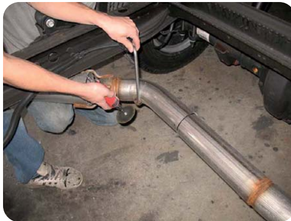
Cut exhaust pipe support on top of the weld as shown on the pic.
