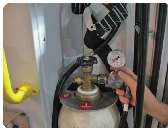
Unplug the oxygen regulator on the main oxygen cylinder.
