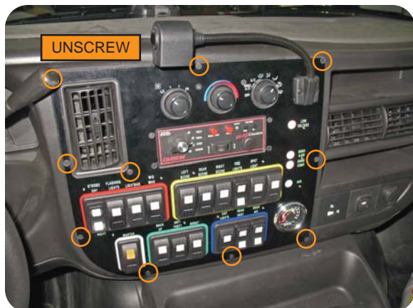
Remove the ten (10) screws.
