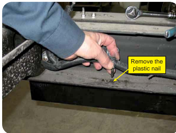
Remove the plastic nail that holds harness in place.
