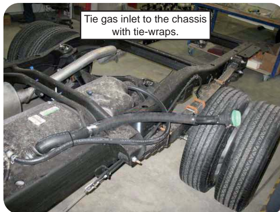
Connect the new pipe with the gas inlet pipe.
