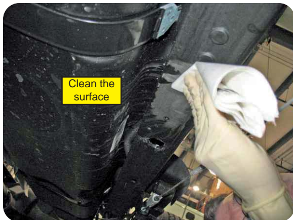
Clean the surface (to rest the drill against).
