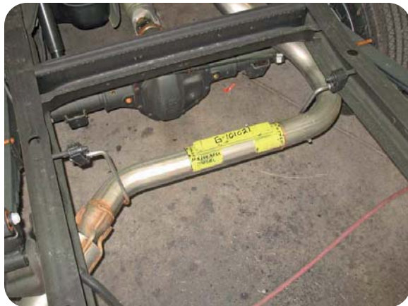
Use jig G-101021 for the exhaust cut out.
