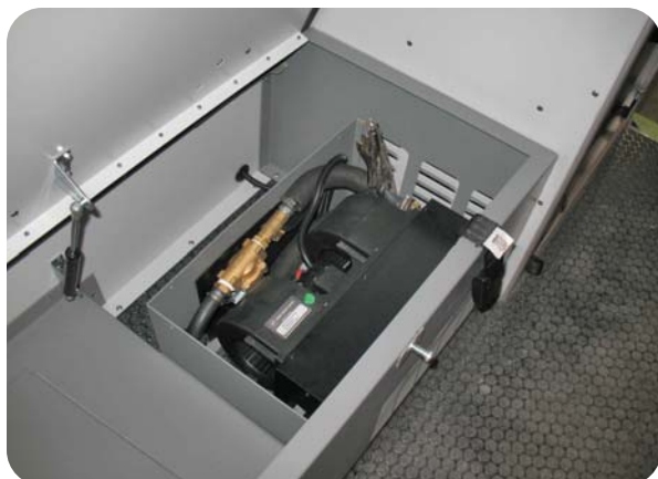
Unplug all hoses and electrical connector and remove (or, if necessary, replace) the standard heating system.
