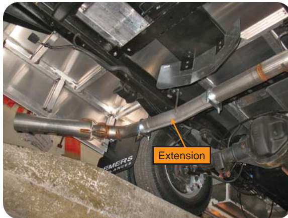
After the module box is installed, install the extension of the exhaust system and fix it with two (2) clamps.
