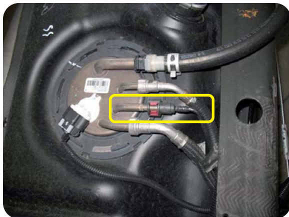
Locate the GM fuel hose as shown on picture.
