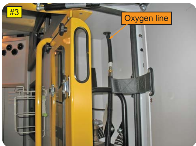
The oxygen line is connected to the main oxygen cylinder, in the patient compartment.
