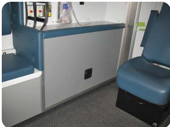
Remove the silicone on all borders of the panel, located under the action wall.
