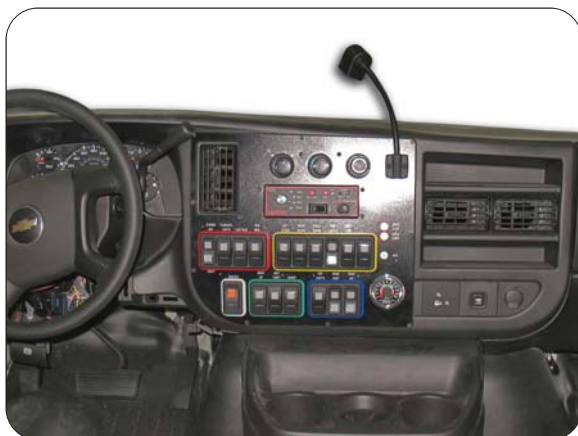
Install the front console.
