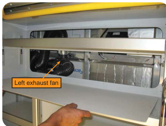
The left exhaust fan is located on the left side of the compartment. To remove the exhaust fan, disconnect first the all vent ducts.
