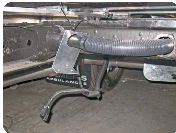
Attach crankshaft conduit to chassis with tie-wrap.
