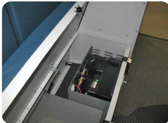
To have access to the standard heating unit, remove the seven (7) screws and remove of the heater protector cover.
