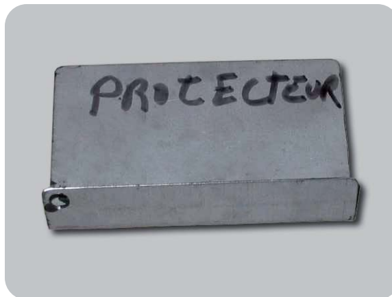
Use a plate to protect the gas tank.
