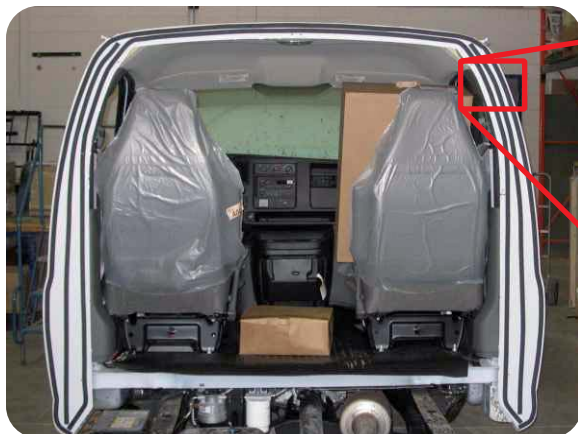
Install the etafoam 1/8" X 3/4" # 204032 on front cabin wall .
