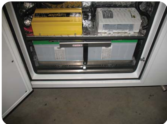
The conversion batteries (the sliding tray closed) in the electrical panel compartment.
