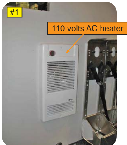
The 110 volts AC heater unit is located on the front wall, in the patient compartment
