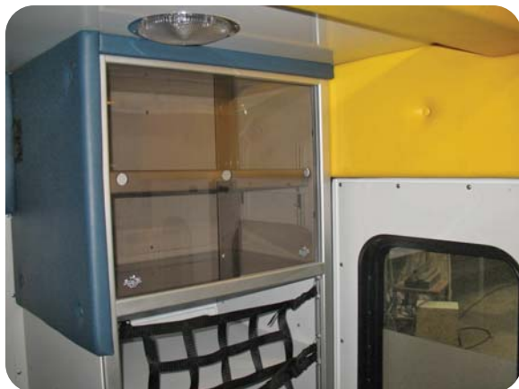
Remove the two (2) cabinet windows.
