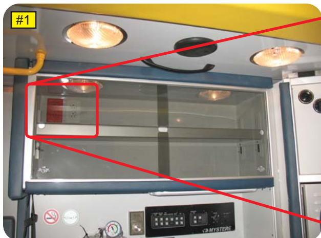
The white 110 volts AC outlet is located on the medical cabinet, in the compartment over action wall.
