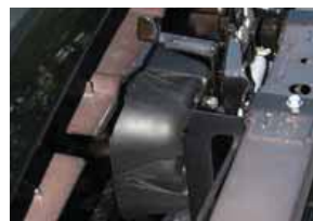
Photo shows mounting placement of SA315P between grille and radiator.
