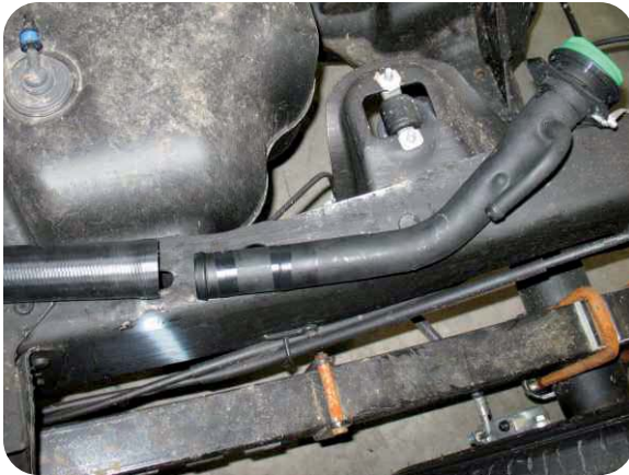
Remove the gas inlet pipe with cap.
