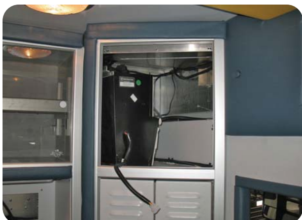
Slowly swivel counterclockwise ( \pm 90^\circ ) the A/C unit.
