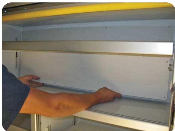
Remove the access panel.
