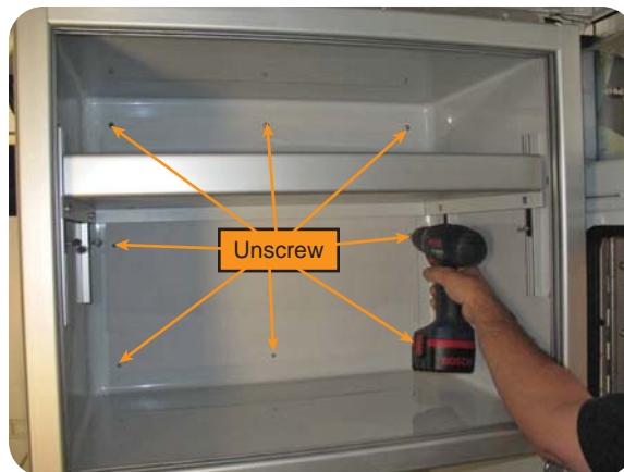
Remove the eight (8) screws.
