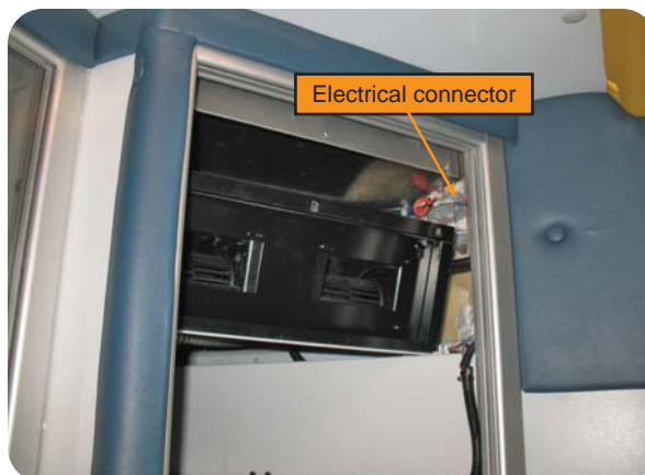
Slowly slide the A/C unit forwards and downwards and disconnect the electrical connector.
