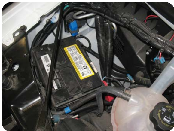
The OEM battery located in the engine compartment.
