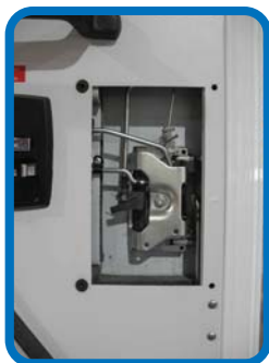
To have access to the mechanism of the door handle.
