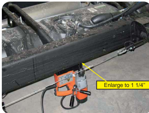
Enlarge the existing hole to 1 1/4"
