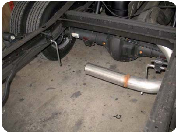
View after the exhaust cut out.
