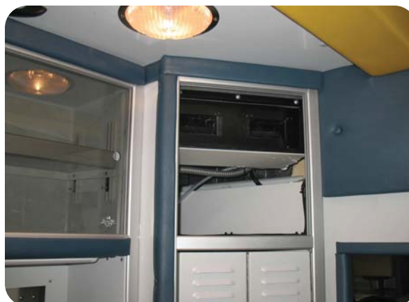
Remove the A/C panel.
