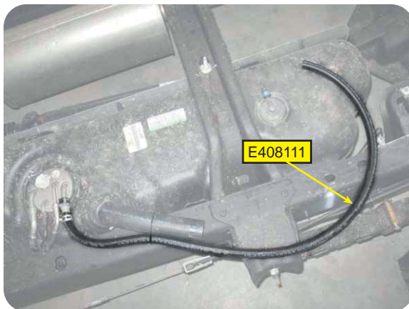
Remove the original vent pipe and install the new pipe (#E408111 X 40"). Reinstall the GM original clamp.
