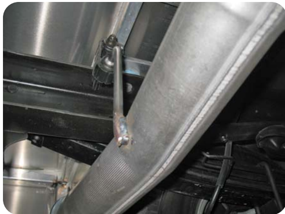
Weld the exhaust pipe support between the GM chassis and the exhaust system extension.
