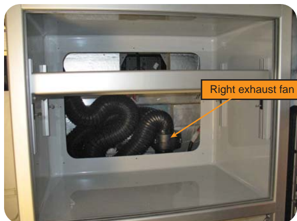
The right exhaust fan is located on the bottom of the compartment. To remove the exhaust fan, disconnect first the all vent ducts.
