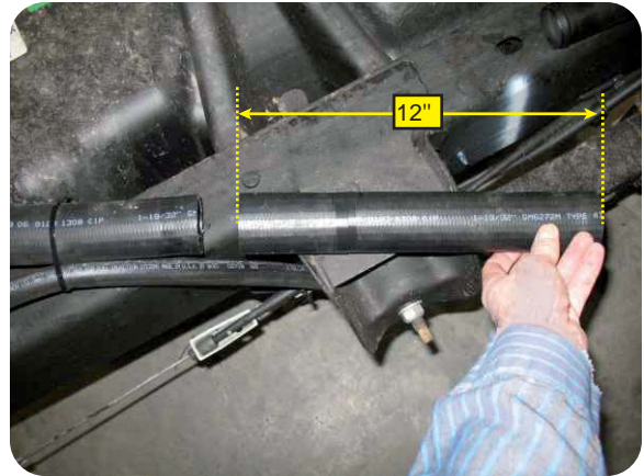
Cut off 12" off the original gas inlet pipe.
