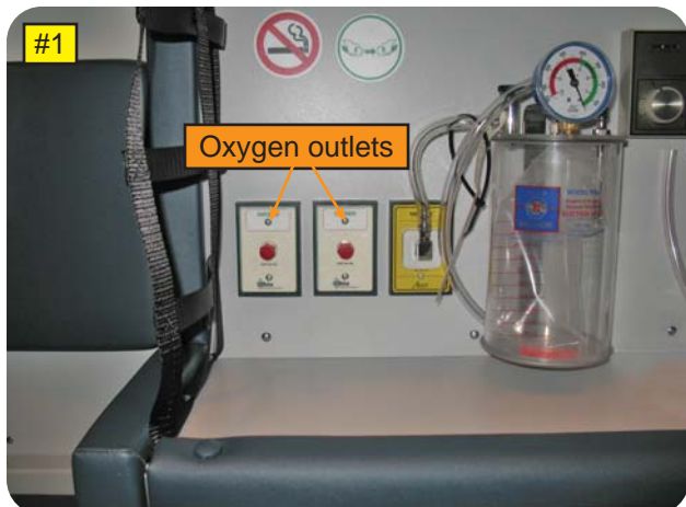
The two (2) oxygen outlets located on the action wall, on the medical cabinet.
