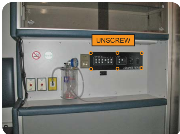
Remove the six (6) screws.
