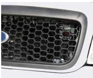
SA315P with vehicle specific mounting in grille of Crown Victoria.
