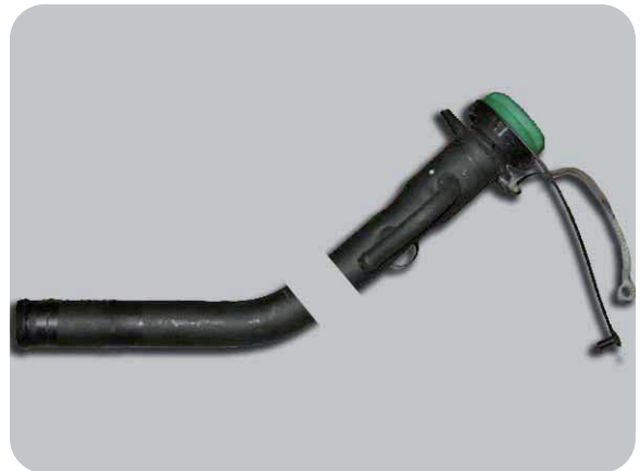
View of modified gas inlet pipe.
